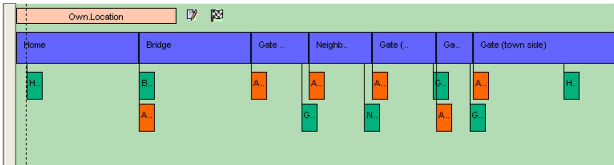
Figure A.7.: A Symbolic-State-Resource which consists of states, like being at home or the bridge .
